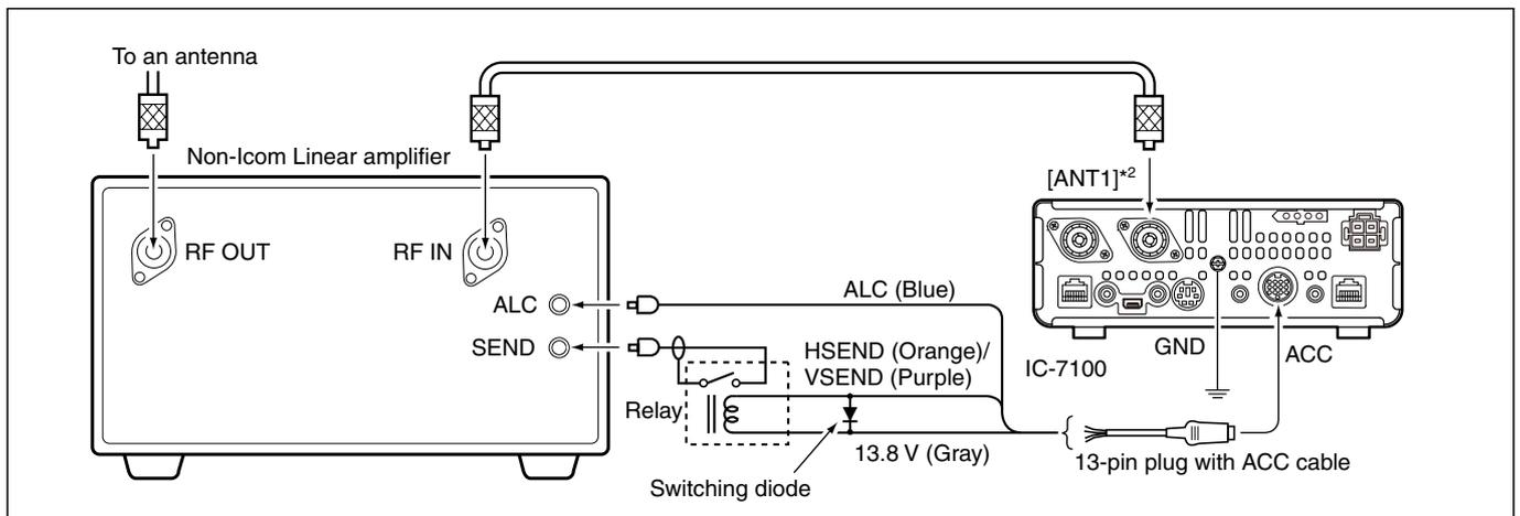
When using a linear amplifier that has a time delay between receiving and transmitting, a high SWR might cause the linear amplifier to malfunction. To prevent this, slow the TX Delay in the "TX Delay (HF), (50M), (144M), (430M)" items of the "Function" Set mode. (p. 6-5)
