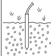
Connect this terminal to a station or vehicle ground to prevent electrical shocks, TVI, BCI and other problems.
