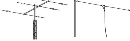
Connect a 50 Ω antenna for the HF, 50/70 MHz frequency bands or below 74.8 MHz.
