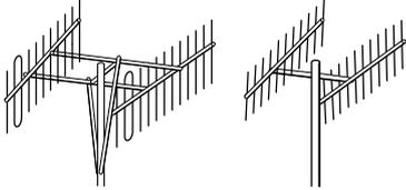
Connect a 50 Ω antenna for the 144/430 MHz frequency bands or 74.8 MHz and above.
