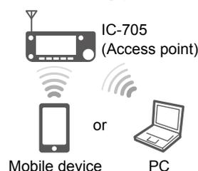
① Only one device can connect to the transceiver at the same time.
