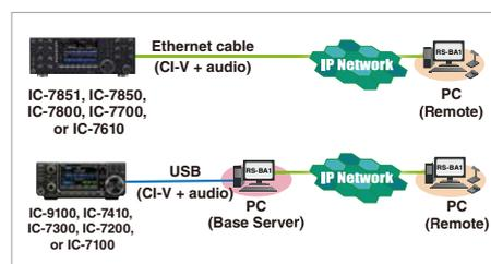
\* A static public IP address (including Dynamic DNS) is required to the base station (Server) PC, when you configure the remote control system through the Internet.
