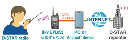
\* The optional free download software, RS-MS3W or RS-MS3A is required to be installed in the PC/Android™ device for terminal mode and access point mode operation. The OPC-2350LU data cable is required.
